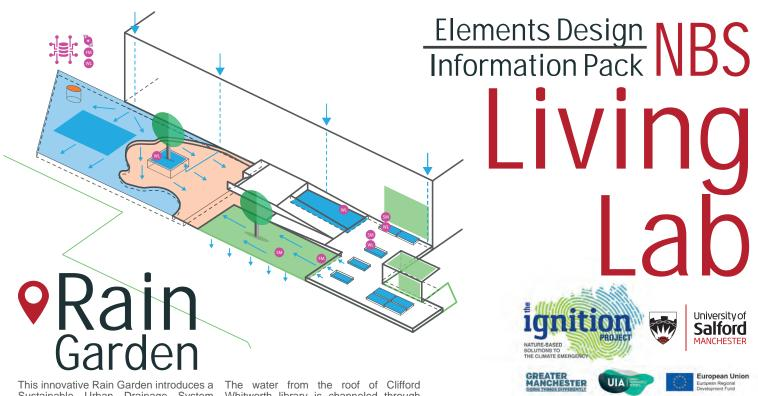
This innovative Rain Garden introduces a Sustainable Urban Drainage System (SuDS) that works as a sequence of passive water management practices, control structures and strategies designed to efficiently and sustainably drain surface water from the adjacent building roof with special regard for engaging biodiversity in the solutions.
