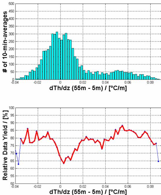
**Figure 1.** Upper panel: Distribution of vertical potential temperature gradient as observed from 2003-05-23 to 2003-07-23. Lower Panel: Percentage of relative data yield of SODAR receptions for the same period, plotted versus pot. temperature gradient.
