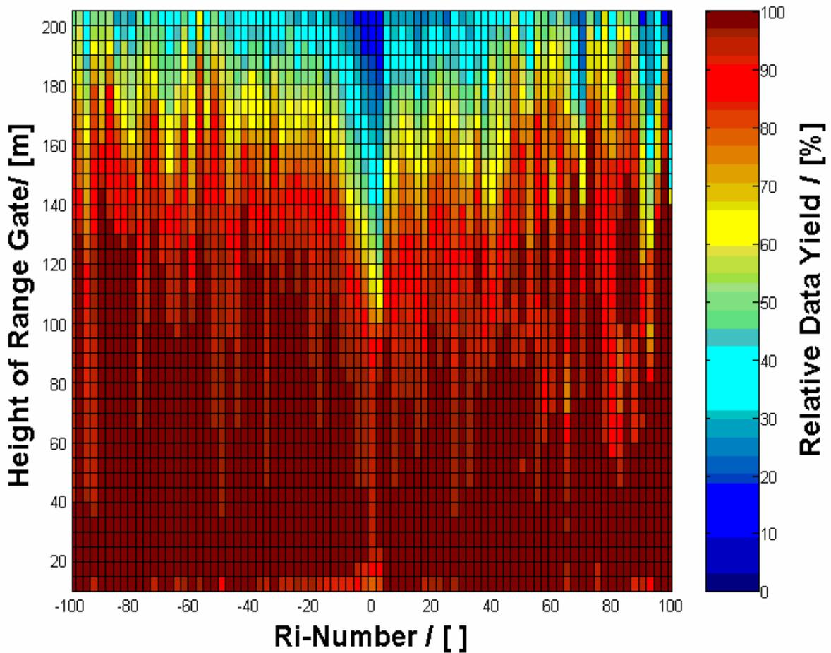
**Figure 3.** Percentage of relative data yield of SODAR receptions as colour map, plotted against height of the SODAR range gates and against the Bulk Richardson number, as calculated from vertical temperature and wind speed gradients, taken from meteorological met mast measurements.
