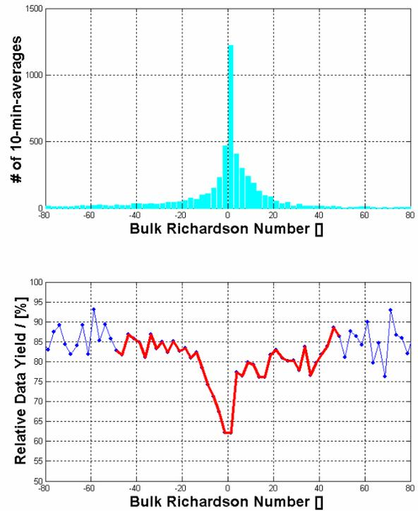
**Figure 2.** Upper panel: Distribution of Bulk Richardson number as observed from 2003-05-23 to 2003-07-23. Lower panel: Percentage of relative data yield of SODAR receptions for the same period, plotted versus the Bulk Richardson number.
